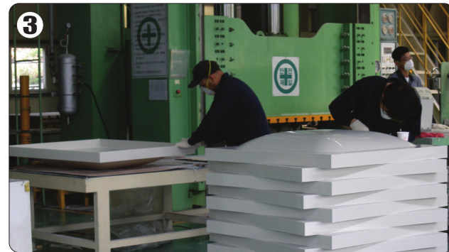
3 Inspect GRP panel
