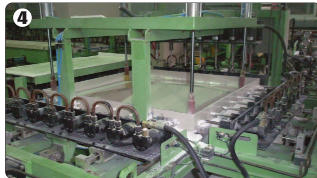
4 Drill on the GRP panel
