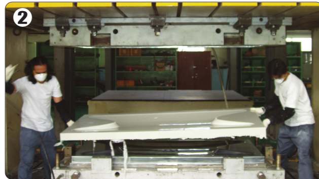
2 Molded by hot hydraulic press
