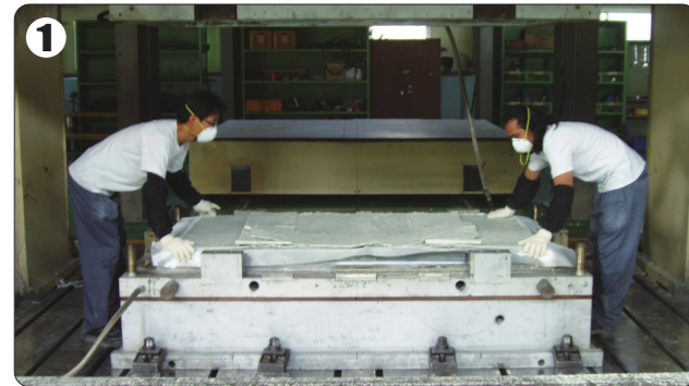
1 Charge SMC sheet on the mould
